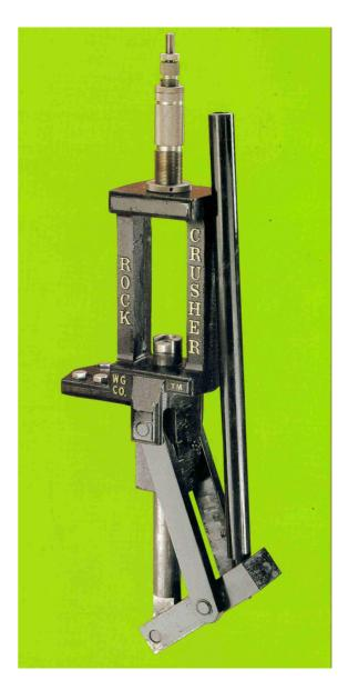
These pictures show a larger calibre reloading press that can be used for calibres up to at least 20mm. Smaller presses can be multistage.
